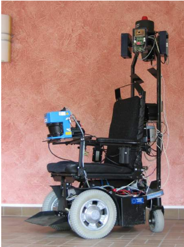
Figure 2.2: The MICA, (Mobile Internet Connected Assistant) wheelchair. An NDC8 navigation system and a camera based navigation system is mounted on top. In the front a SICK LMS200 range measuring laser is seen.
