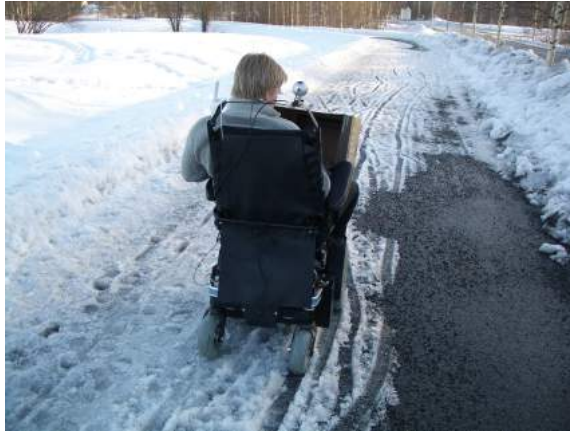
Figure 13: The robot driving autonomously through snow slush on a plowed walking path in the campus area.
