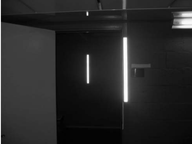
Figure 1: In the figure two retroreflective beacons at different distances are visible, the one to the left is at app. 6m and the one to the right is at app. 3m distance. The width of the beacons is 36mm and the height is 750mm. The picture is taken with an ordinary digital camera with a built in flash.
