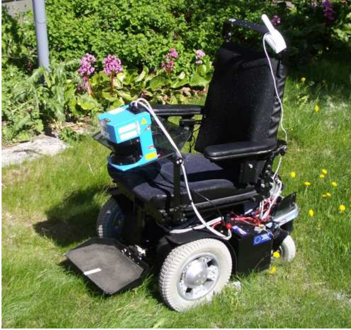
Figure 9: The wheelchair used in the tests. It is equipped with a pitched range scanning laser, a rate gyro and two wheel-encoders. It carries an embedded x86 computer running RedHat Linux 7.3 which is used to collect and time stamp sensor readings. It controls the wheelchair. Clients can connect to the on-board computer over a wireless link and request sensor readings and send control commands. Using the implemented circle sector expansion method, the wheelchair was able to explore an unknown environment using the MATLAB environment on a standard Laptop computer running Windows-XP.
