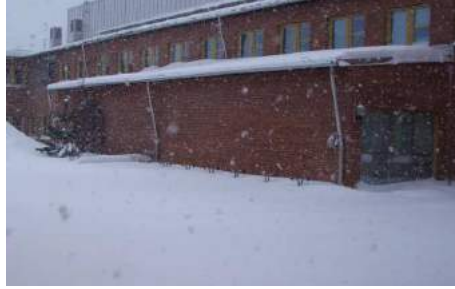
Figure 14: A part of this wall was used as reference object to get statistics about percentage of false detections by snowflakes, detections on the object behind, and no detections. It is possible to see falling snowflakes in the picture.
