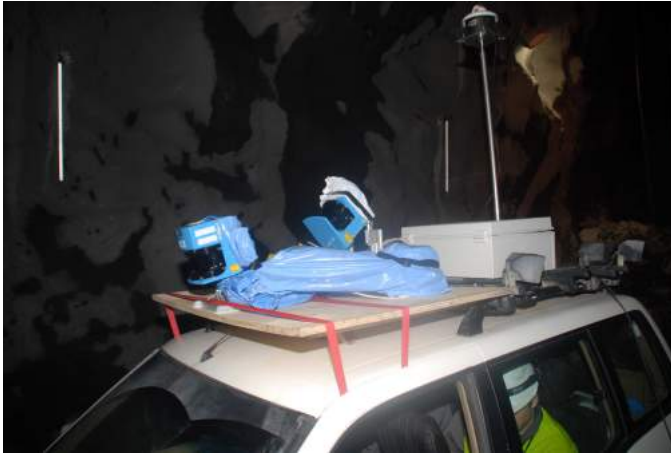
Figure 3.1: Test setup used when collecting measurements in the LKAB underground mine in Kiruna, Sweden. For navigation, we used an NDC8 system. The navigation laser is visible on top of the long stick on the rear part of the car. Two retroreflective beacons are also visible on the wall in the background. As environmental sensors we used two SICK LMS200 laser scanners. One of the lasers is tilted looking down on the ground and one is tilted up towards the ceiling.
