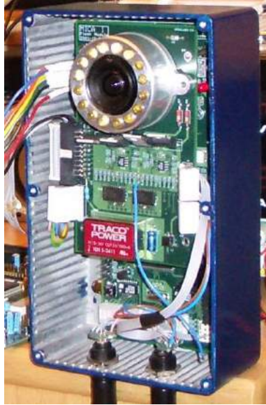
Figure 2: An ordinary LED flash consisting of 16 Light Emitting Diodes mounted in a circle around the camera lens. All LEDs are placed at equal distance from the optical axis of the camera. The flash is mounted on a CMOS camera based navigation system prototype.
