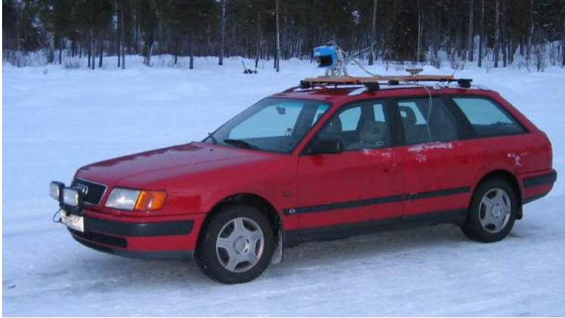
Figure 1: Testcar on a frozen lake used as an icetrack for automobile testing under arctic conditions. The laser sensor, tilted downwards, and a GPS antenna are mounted on the roofrack of the car.
