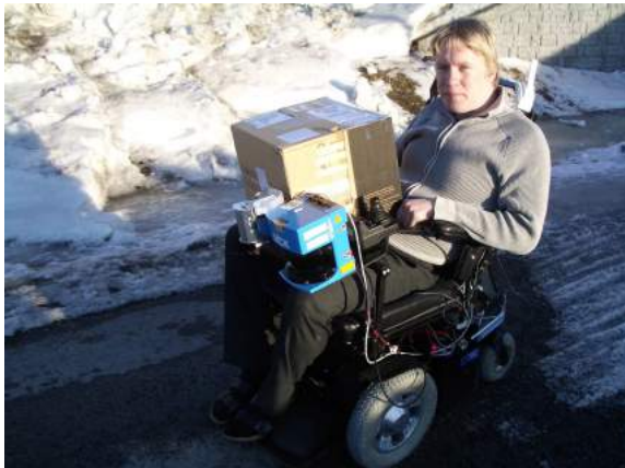
Figure 11: Robot used as platform during the closed loop testing. The LMS200 laser is seen in the front, the box behind it is a sunscreen for a laptop. The only function of the person is emergency stopping.
