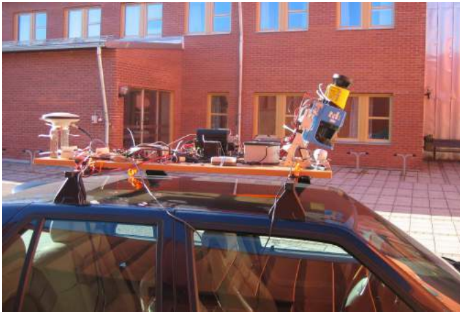
Figure 3.2: Test setup used during the measurements at a gokart track in Luleå, Sweden. All sensors and all other necessary equipment are placed on the plate on the roof rack. For navigation during the test, we used a NovAtel SPAN system consisting of a GPS receiver with an external IMU. Two different range measuring lasers - one SICK LMS200 and one SICK S300 - are mounted on top of each other, both looking forward and tilted down to see the ground.
