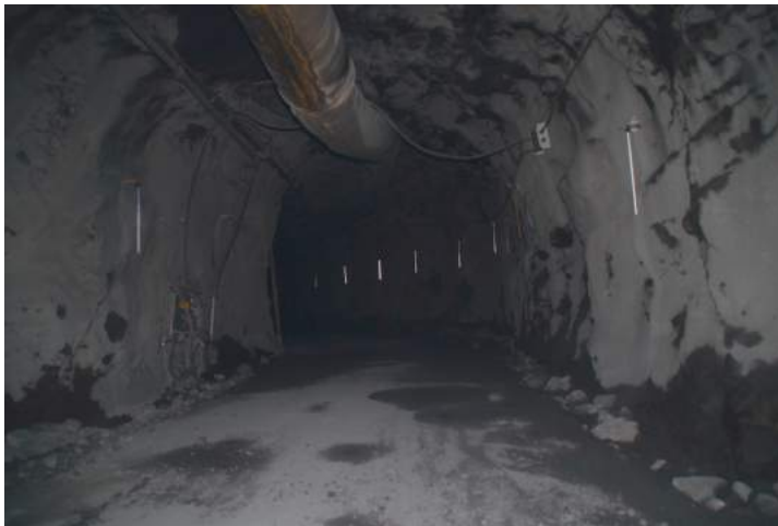
Figure 2.1: Picture from the LKAB underground mine in Kiruna, Sweden. On both sides of the tunnel one can see the retroreflective beacons used by the navigation system on the autonomous LHD vehicles.
