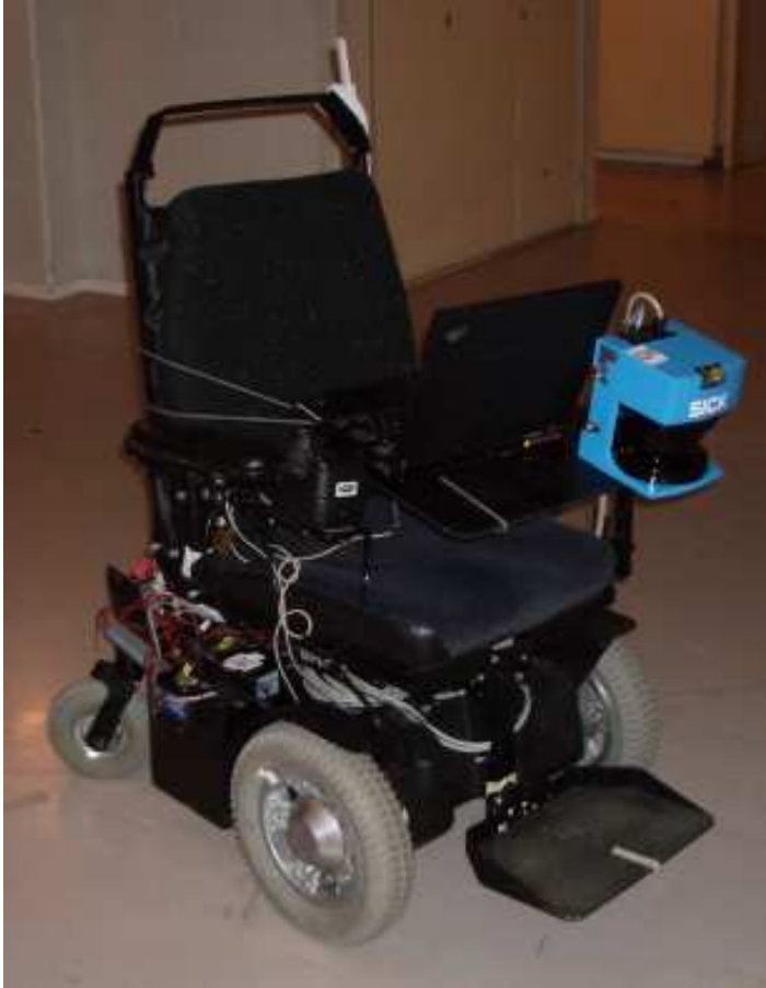
Figure 9: We used a modern wheelchair equipped with a SICK laser for the tests. The laser is pitched down approximately 4^\circ . It is also equipped with an embedded PC computer that runs a software that collects and time stamps sensor data readings. The computer is accessible over W-LAN, the antenna is visible on the top of the wheelchair. The used fiber optic gyro is visible under the seat between the front and back wheel.
