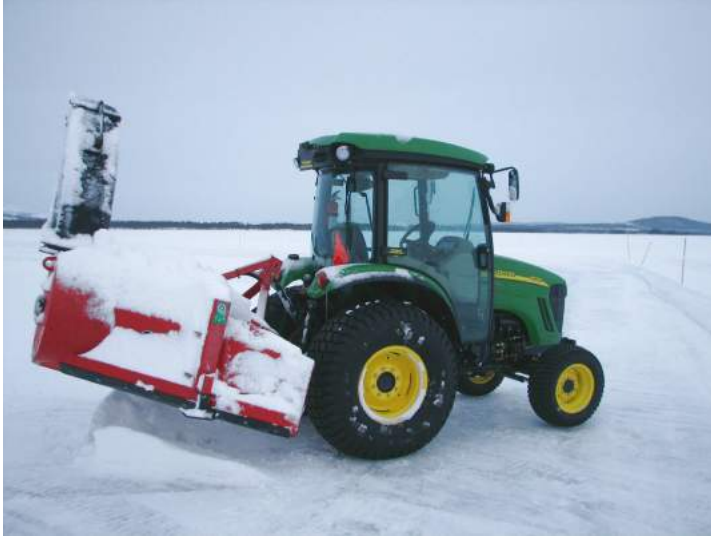
Figure 3.4: IceMaker I, a tractor with mounted snow blower in its natural frozen lake environment. Its purpose is to remove snow. The tractor is part of a research project at Luleå University of Technology.
