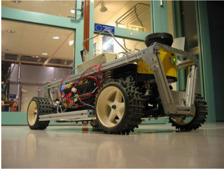
Figure 3.3: MiniLusar is a scale 1:5 RC-car. It was originally petrol driven, but it has been converted to electrical drive to enable indoor use. It is, apart from batteries and necessary servos for controlling it, equipped with a rate gyro, a laser scanner, and a computer with WLAN access.
